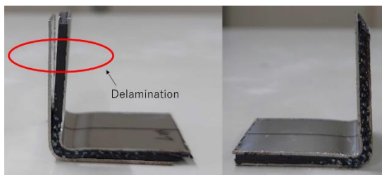
P (Stainless steel/CFRTP) A (Aluminum alloy/CFRTP) Fig. 3 Photographs of specimen
