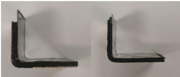
(a) Aluminum/CFRTP (b) Stainless /CFRTP
