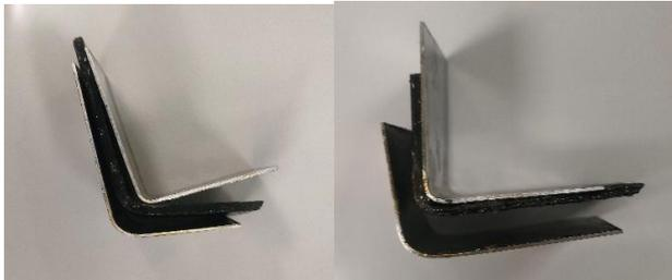
(a) Aluminum/CFRTP (b) Stainless /CFRTP
