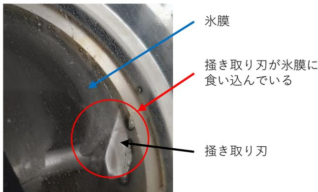
Fig. 4 Generator immediately after  $180\text{min}^{-1}$  Measurement
