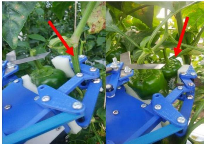
Fig 2.2 Failure to harvest green bell peppers <sup>(7)</sup>
