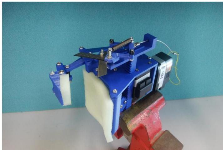
Fig 2.1 Picking mechanism <sup>(7)</sup>
