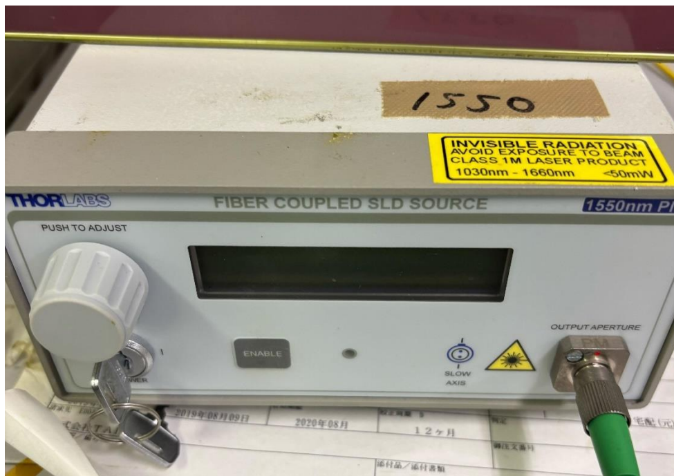
Fig. 5.1.2 SLD light source (1550nm, Thorlabs)
