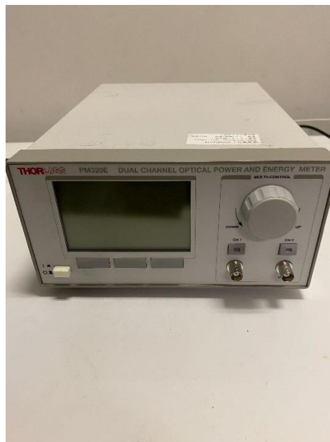
Fig.4.1.6 Optical power meter (PM320E, Thorlabs)
