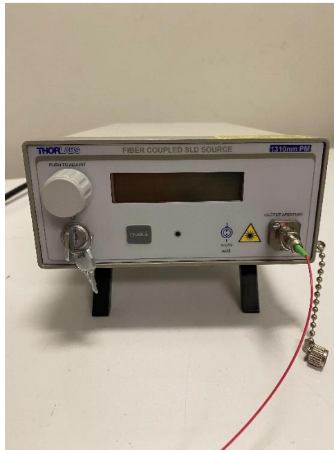
Fig.4.1.5 SLD light source (S5FC1021S,1310nm, Thorlabs)
