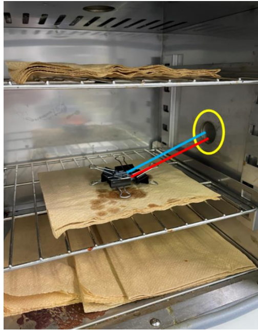
Fig.4.1.9 Experimental set-up measurement of refractive index change in the oven
