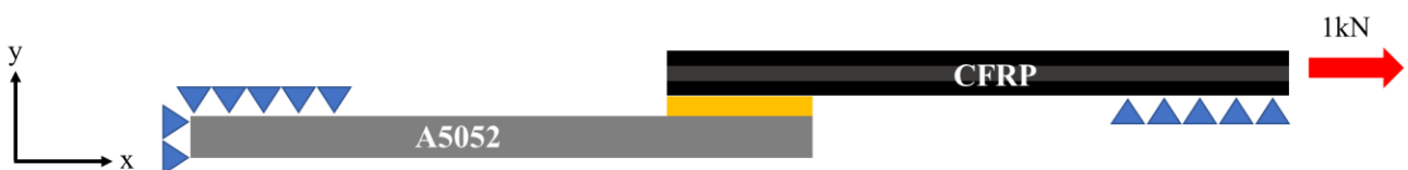
Fig. 27 Configurations of the SLJ test piece (mm)
