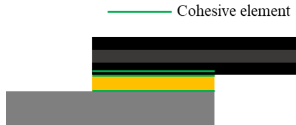
Fig. 31 Cohesive element in the adhesive joint
