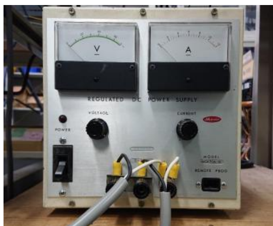
Fig. 4.6 DC power supply
