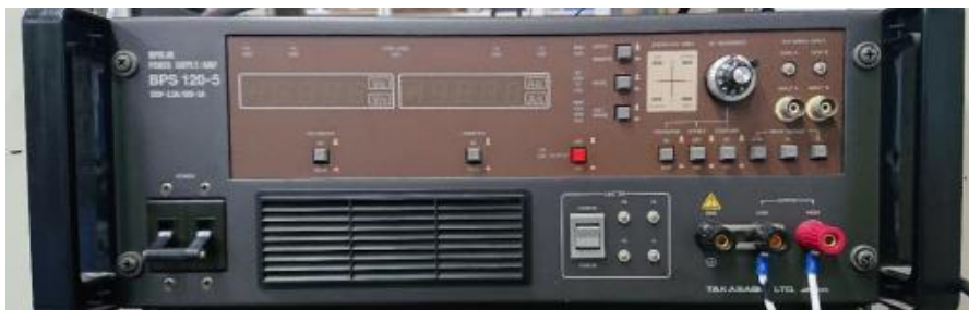
Fig. 4.7 Power amplifier for Contact-less power supply
