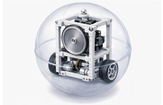
Fig.1 Structure model of the spherical rover
