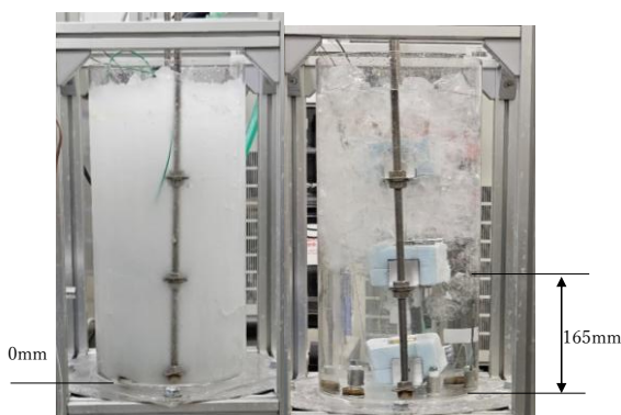
Fig.4 Appearance of slurry ice and ice water immediately after the start of measurement ( IPF=30\% )
