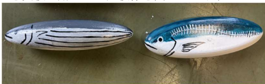
Fig. 3-1 Test specimens with fusiform morphology (left) and flattened morphology (right)
