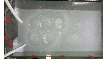
Fig. 5-2 Bubbling behavior with 4mm outlet diameter and 85L/min flow rate
