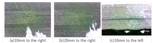
Fig.3 State of delamination
